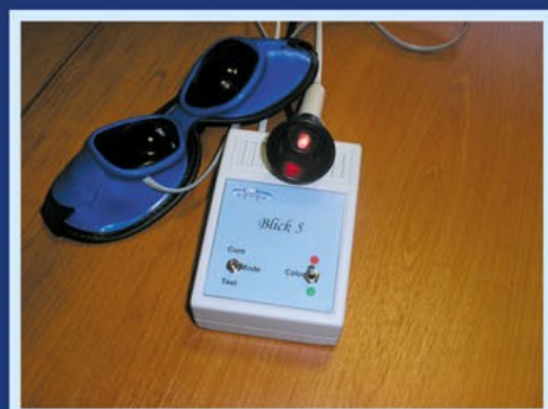
Fig. 2. A device for measuring critical flicker-fusion frequency (CFF) to color stimuli (red, blue and green) – Blick 5. Frequency of light stimulus flickers: 5– 60 Hz Frequency variation step: 0.5 Hz Maximum power of the light pulse: 0.8 micro candles Light diodes: red, blue, green
