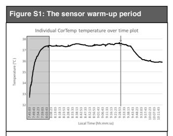
The figure represents a section of the raw CorTemp data plot for participant number fourteen. The grey arrows indicate the time of spinal anesthetic injection at 09:29:00. After ingestion the CorTemp sensor requires time to warm up to the surrounding tissue temperature. For each participant the warm-up period (grey shaded area) was identified by visual inspection and cut from the CorTemp data prior to statistical analysis.
