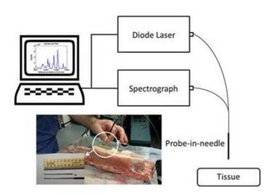
Supplemental Figure 2. The probe-based tissue spectroscopy setup for in-situ measurements. Raman spectra were acquired while inserting the needle from epi-/dermis to spinal cord. A 2 mm outer diameter Raman probe is integrated into the 2 mm inner diameter custom short bevel needle and Raman spectra were collected at the tip of the needle.
