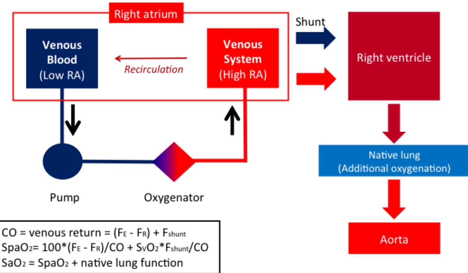
**Supplemental Figure 1.** Physiological determinants of oxygenation in femoro-jugular configuration of venovenous extracorporeal life support (ECLS). Shunt flow ( $F_{\text{shunt}}$ ) is the blood flow that bypasses the ECLS circuit. CO: cardiac output;  $F_E$ : ECLS flow;  $F_R$ : recirculation;  $SpaO_2$ : pulmonary arterial oxygen saturation;  $SaO_2$ : arterial oxygen saturation.
