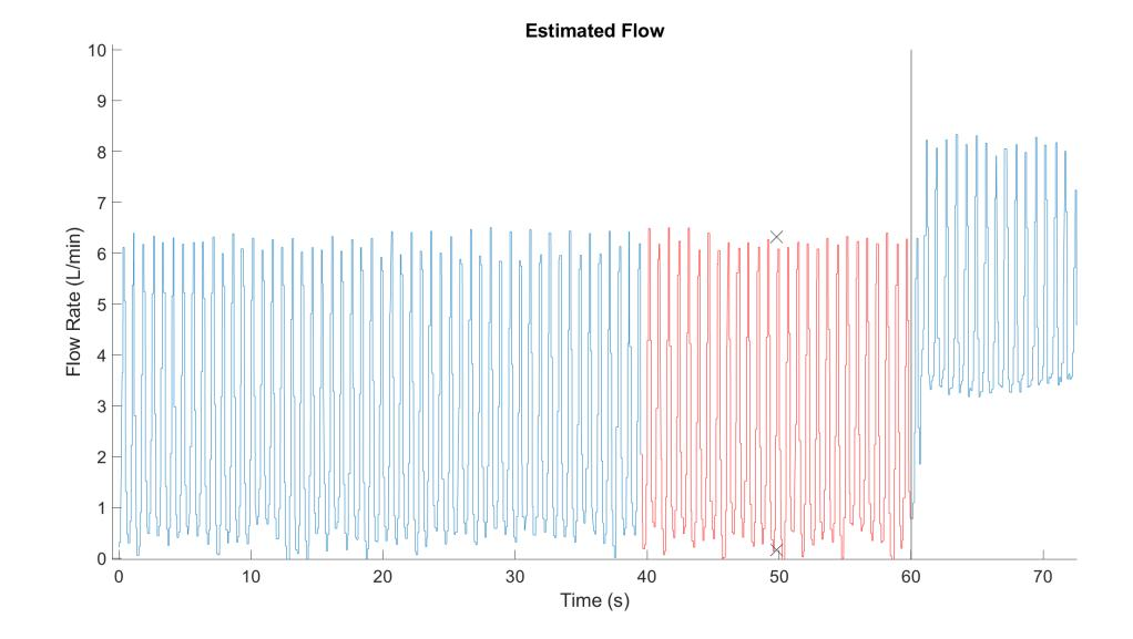
An example showing the instantaneous estimated waveform (blue) and the portion of the waveform analysed by the peak and trough detector (red). The average peaks and trough levels are given by the black crosses
