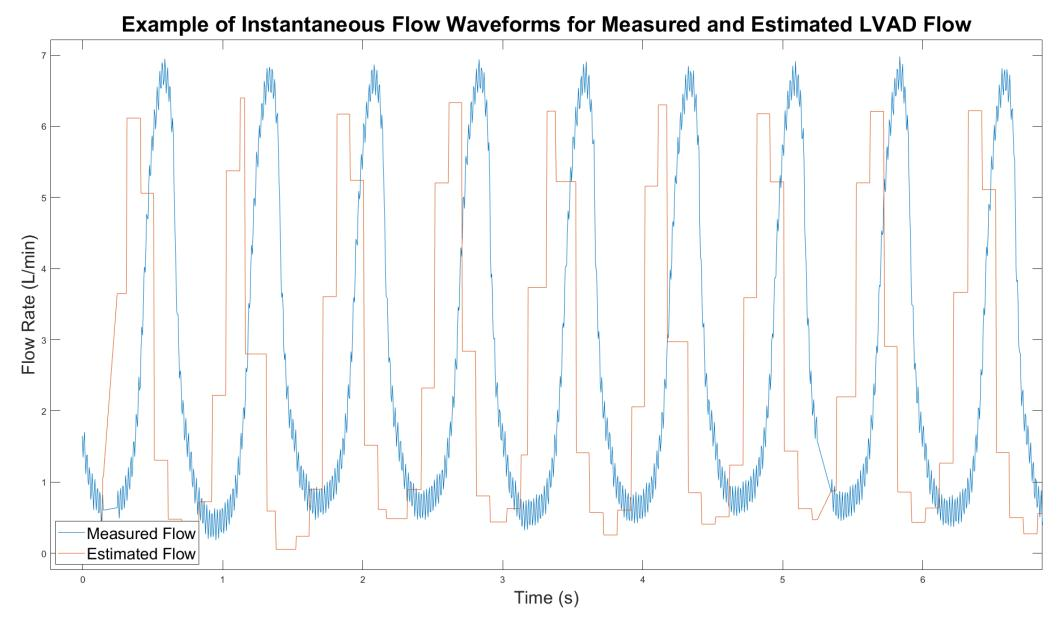
An example of the raw instantaneous flow waveforms for measured and estimated LVAD flow at 80 beats per minute, SVR 1300, PVR 100, CVP 12, LVAD speed 2500 rpm. Note the sampling rate is the same between the two signals, but the estimated signal updated from the controller at a lower frequency ~ 20 Hz
