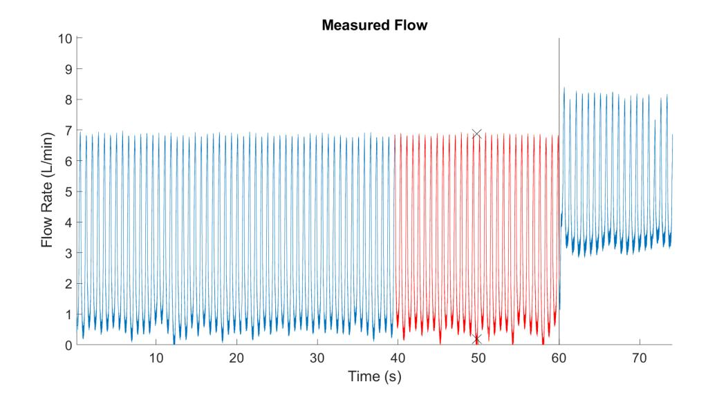
An example showing the instantaneous measured waveform (blue) and the portion of the waveform analysed by the peak and trough detector (red). The average peaks and trough levels are given by the black crosses
