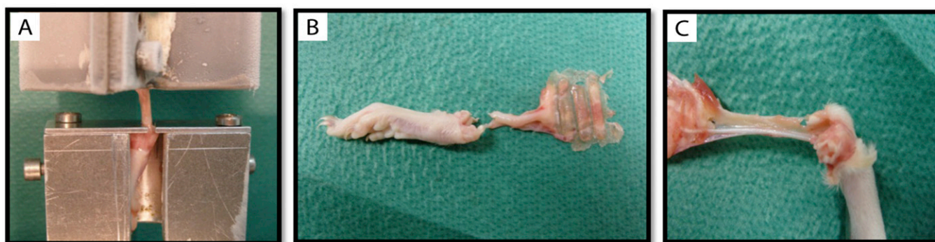
Fig. E-2 Figs. E-2A, 2-B, and 2-C Biomechanical testing. Fig. E-2A Biomechanical testing with proximal cryoclamp fixation and the distal mounting grid with osseous calcaneal fixation. Figs. E-2B and E-2C Tendon after load to failure testing.
