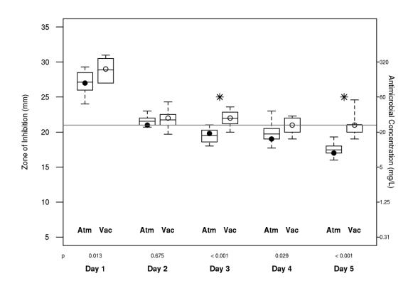
Average zone of bacterial growth inhibition (left) and antimicrobial concentration (right) for atmospheric (Atm; solid circles) and vacuum-mixed (Vac; open circles) Palacos R+G. The horizontal line represents the 32-mg/L susceptibility threshold. \*The difference was significant. The boxes represent the first and third quartiles, the horizontal lines within the boxes represent the median, and the I-bars represent the 5th and 95th percentiles of the data.
