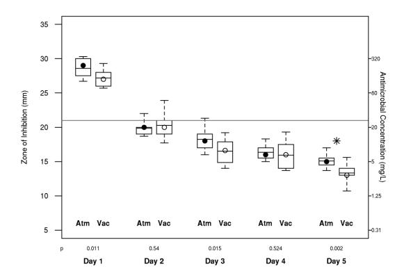
Average zone of bacterial growth inhibition (left) and antimicrobial concentration (right) for atmospheric (Atm; solid circles) and vacuum-mixed (Vac; open circles) VersaBond AB. The horizontal line represents the 32-mg/L susceptibility threshold. \*The difference was significant. The boxes represent the first and third quartiles, the horizontal lines within the boxes represent the median, and the I-bars represent the 5th and 95th percentiles of the data.
