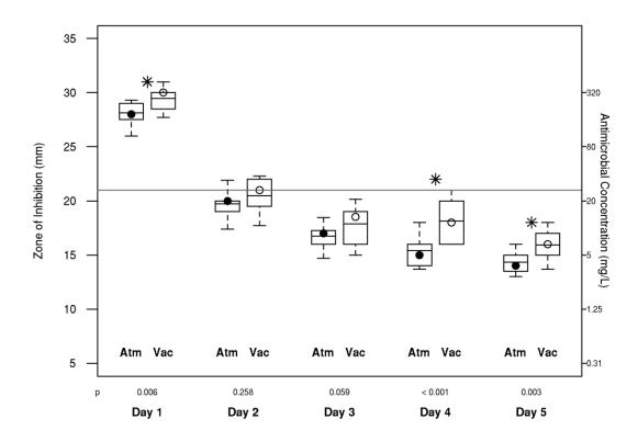
Average zone of bacterial growth inhibition (left) and antimicrobial concentration (right) for atmospheric (Atm; solid circles) and vacuum-mixed (Vac; open circles) Simplex P with Tobramycin. The horizontal line represents the 32-mg/L susceptibility threshold. \*The difference was significant. The boxes represent the first and third quartiles, the horizontal lines within the boxes represent the median, and the I-bars represent the 5th and 95th percentiles of the data.
