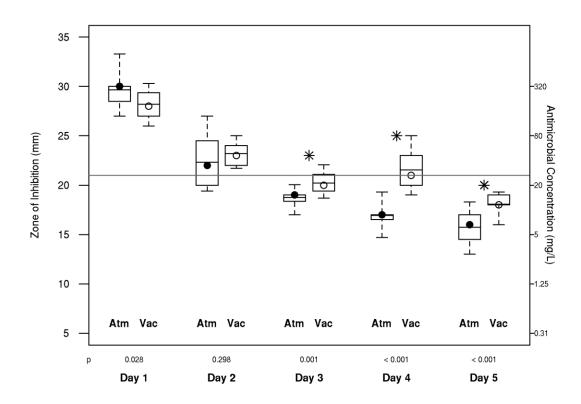
Average zone of bacterial growth inhibition (left) and antimicrobial concentration (right) for atmospheric (Atm; solid circles) and vacuum-mixed (Vac; open circles) Cobalt G-HV. The horizontal line represents the 32-mg/L susceptibility threshold. \*The difference was significant. The boxes represent the first and third quartiles, the horizontal line within the boxes represents the median, and the I-bars represent the 5th and 95th percentiles of the data.
