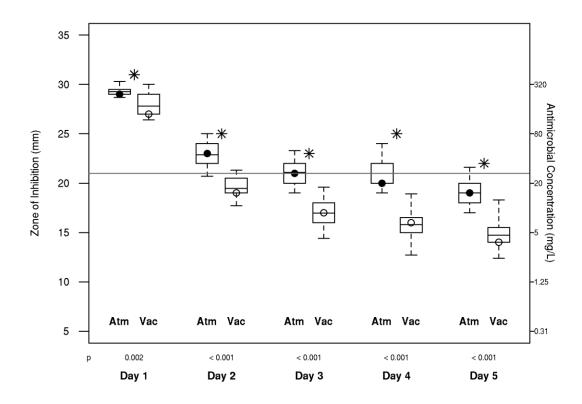
Average zone of bacterial growth inhibition (left) and antimicrobial concentration (right) for atmospheric (Atm; solid circles) and vacuum-mixed (Vac; open circles) Cemex Genta. The horizontal line represents the 32-mg/L susceptibility threshold. \*The difference was significant. The boxes represent the first and third quartiles, the horizontal line within the boxes represents the median, and the I-bars represent the 5th and 95th percentiles of the data.
