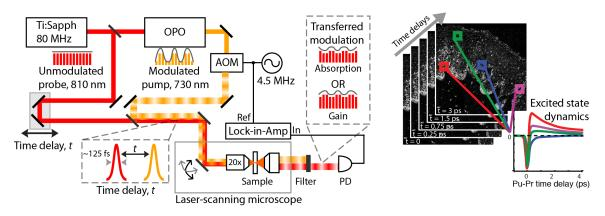
Figure S1: System schematic and data acquisition. Ti:Sapph: Titanium-Sapphire laser. OPO: Optical Parametric Oscillator. AOM: Acousto-Optic Modulator. PD: Photodiode.
