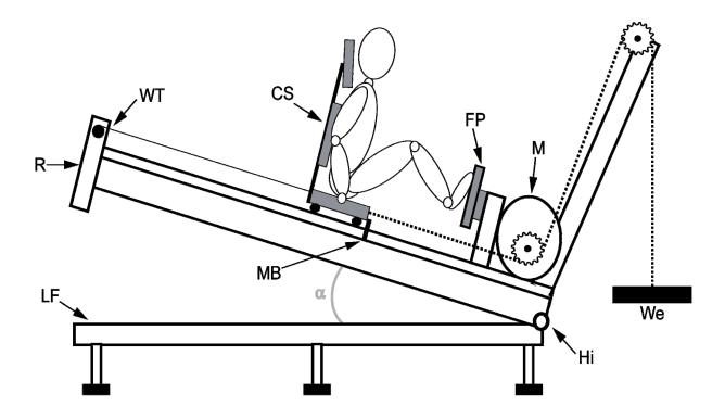
Schematic view of the Explosive Ergometer (EXER). WT wire tachometer, CS carriage seat, FP force platforms, M electric motor. Rail system (R) and lower frame (LF) are hinged (Hi) so that R can be tilted upward (see text for further details). To allow the motor to act on the seat without delays, a constant tension (We = 196 N) is applied to the steel chain (dotted line).
