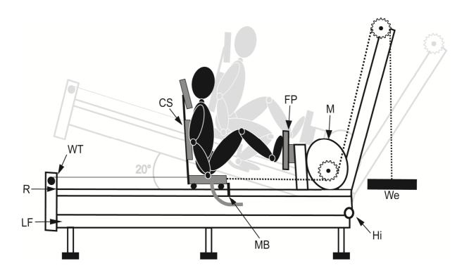
Schematic views of the Explosive Ergometer (EXER) for horizontal or inclined lower limb extensions in bilateral and unilateral conditions. WT wire tachometer, CS carriage seat, FP force platforms, M electric motor, MB mechanical block. Rail system (R) and lower frame (LF) are hinged (Hi) so that R can be tilted upward. To allow the motor to act on the seat via the chain without delays, a constant tension (We = 196 N) is applied to the steel chain (dotted line) (see 26).
