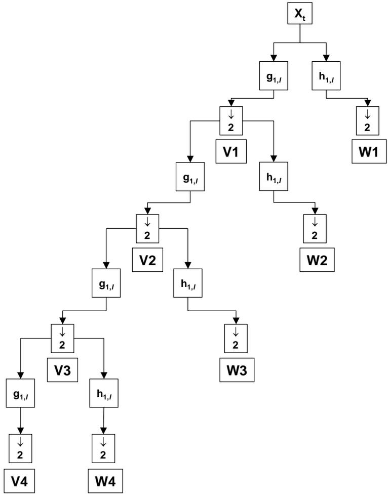
Fig. 3. The successive filtering with the wavelet and the scaling filter, shown as a pyramidal filter bank for a multi resolution analysis down to scale 4.
