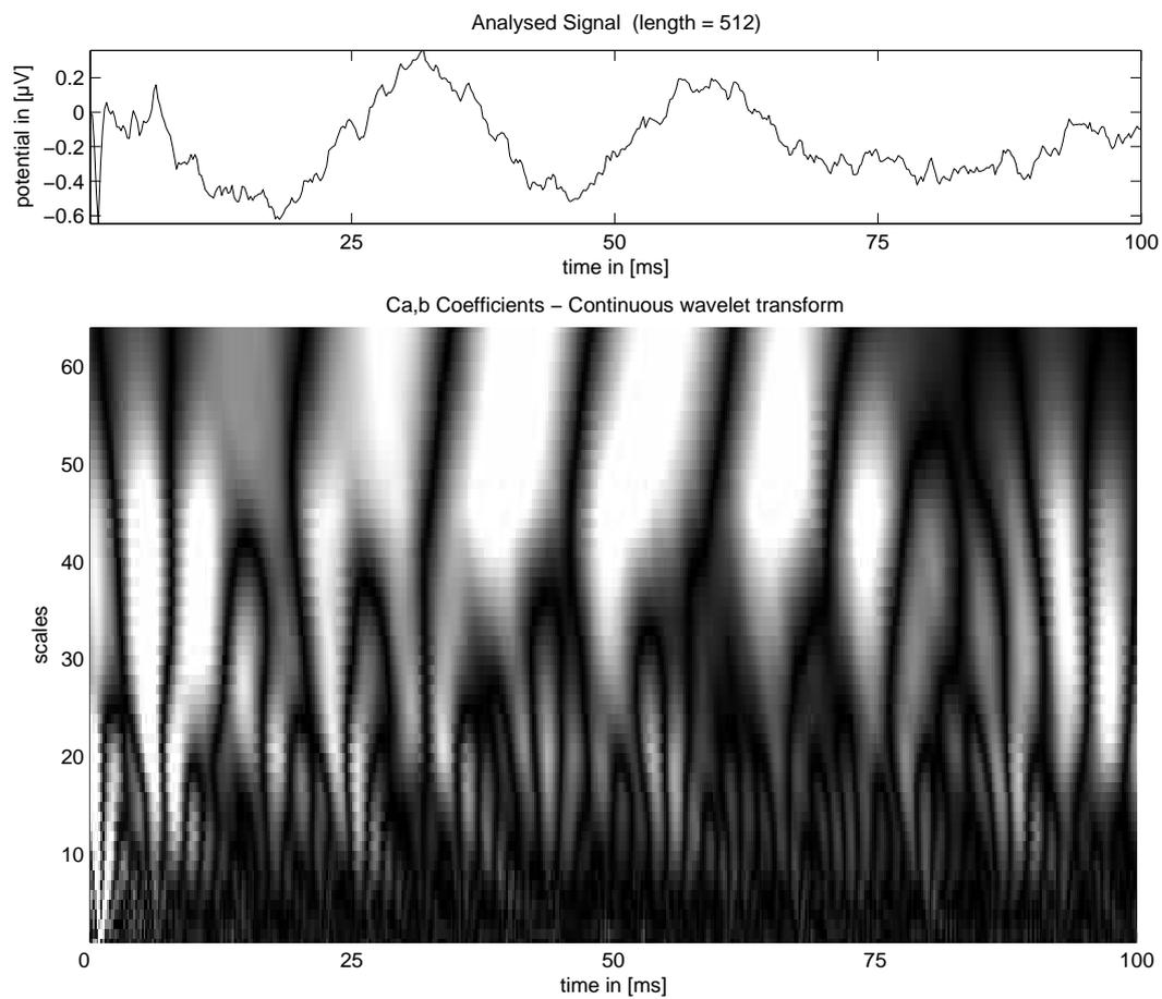
Fig. 2. Continuous wavelet transform of an auditory evoked potential sampled at 5120 Hz with the Daubechies 4 Wavelet on 64 scales.
