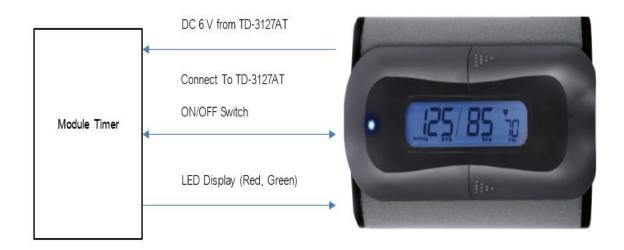
Instruction on how to install the Timer Module to the TD-3127AT Pressure Gauge. The module is installed inside the pressure gauge by
