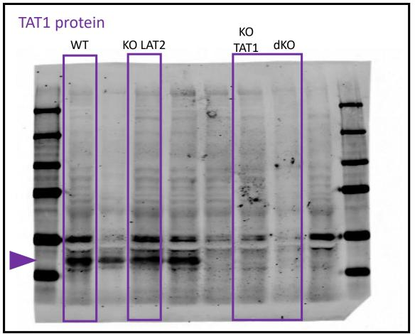
First and last lane in both gels is for molecular weight marker, corresponding to 220, 150, 100, 75, 50 and 37 kDa bands.
